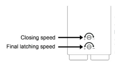
To adjust, turn both screws clockwise until they stop. This will mean the gate will be locked in position. Then undo until they are the correct speed ensuring they do not turn more than 3 full turns from the stopped position
